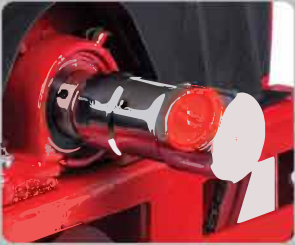
Water Inlet Bearing with 1" Crom Marble Bedding
